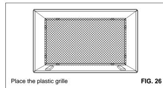
**3** Fasten the 4 washer screws to secure the grille to the wall sleeve. If you need plastic nuts to mount plastic grille to the inside of the wall sleeve, there are plastic nuts in the installation kit. The nuts are installed from the inside of the sleeve and are pressed into the square holes of the rear flanges.
